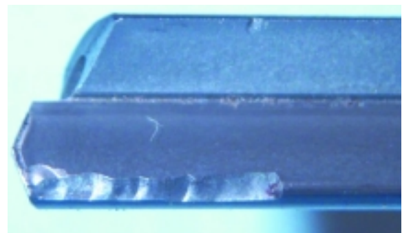
Figure 4: Excessive clearance between the starting bushing and drill tip can cause edge breakage.
