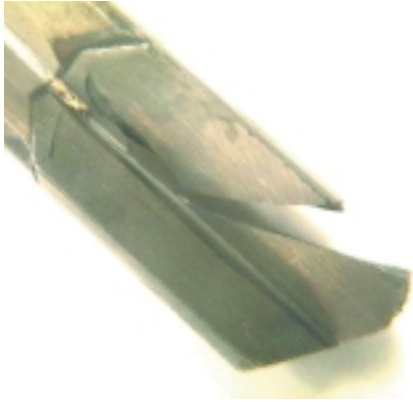
Figure 2: Drill failure as a result of excessive misalignment between the starting bushing and machine spindle.
